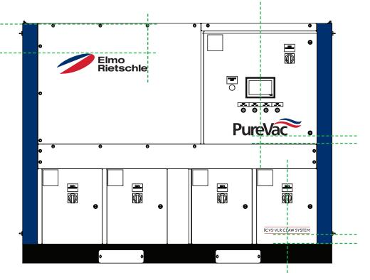
System model decal is centered on the lower-right panel, approximately 2.6" away from the bottom edge of the panel.
